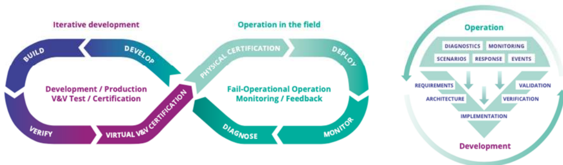
Figure 2.3.2 Simplified examples for continuous development processes (DevOps processes). Such processes are essential for building future ECS-based systems and products since they enable data collected during the operation phase to be used in iterative (continuous) development for updates of existing products.
